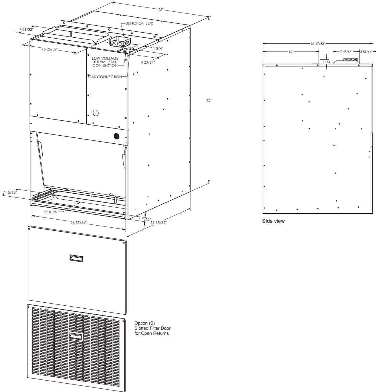
NOTE: Unit must be mounted a minimum of 8 inches above finished floor.
