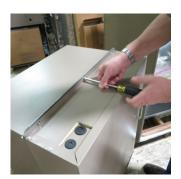
The Insulated Sound Cover will be supplied insulated, handles installed and assembled. To install on to the unit, either the top or bottom will need to be removed, depending, on the exit point, of the tubing. (4 screws)
