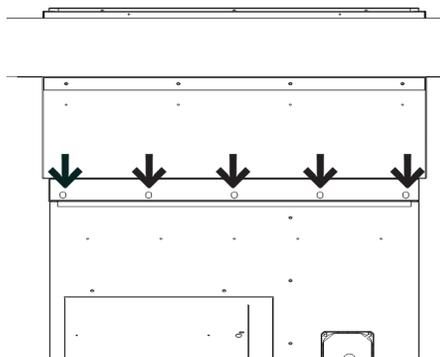
**NOTE: FOR EASE OF INSTALLATION, INSTALL THE CABINET INTO THE WALL SLEEVE FIRST WITHOUT THE COOLING CHASSIS. THEN SLIDE COOLING CHASSIS IN AFTER CABINET IS IN PLACE.**
