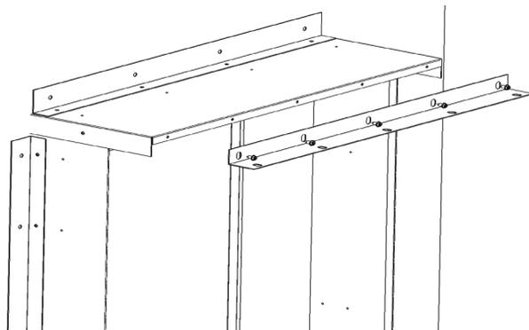
Slide the unit into the wall sleeve and fasten the unit to the sleeve with the five screws provided with the sleeve.
