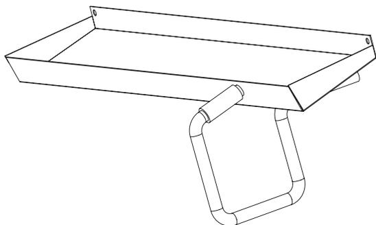
4. Position the trap as shown and slide the 2" piece of clear flexible tubing about 1" onto the top end of the trap. Slide the top of the flexible tube on the trap onto the bottom of the 1/2" OD secondary drain connection and push the top of the trap up.
