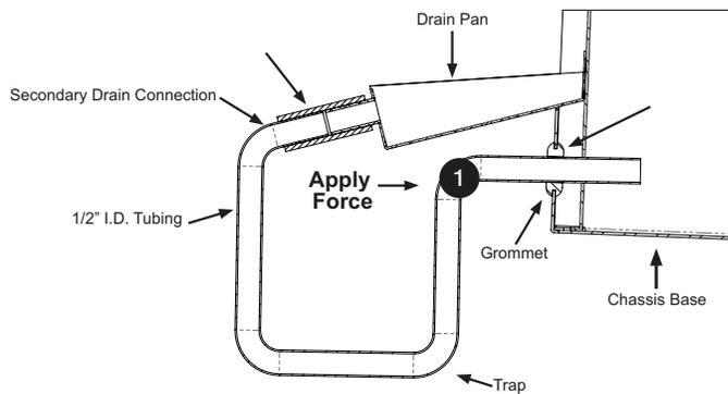
The trap should be positioned so that there is only a small gap between the top of the trap and the bottom of the secondary drain connection.
