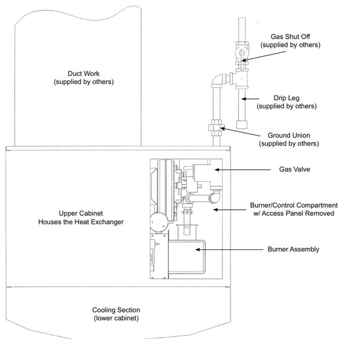
\*Install the heat exchanger inspection panel in the ductwork in such a manner that will prevent air leaks.
