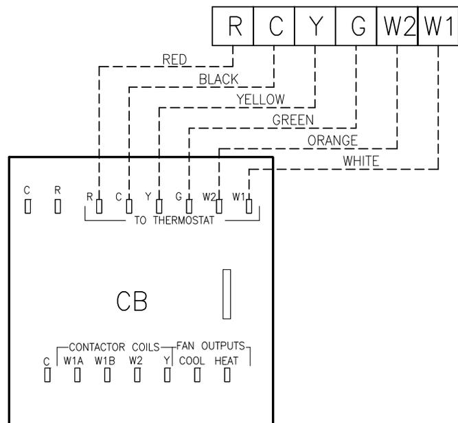
**NOTE: IF A 2 STAGE THERMOSTAT IS NOT USED CONNECT BOTH WHITE(W1) AND ORANGE(W2) WIRES TOGETHER. THESE WIRES ARE ONLY NEEDED ON COMFORT PACKS INSTALLED WITH CPEHK**
