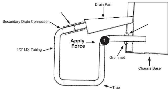
4. Position the trap as shown and slide the 2" piece of clear flexible tubing about 1" onto the top end of the trap. Slide the top of the flexible tube on the trap onto the bottom of the 1/2" OD secondary drain connection and push the top of the trap up. The trap should be positioned so that there is only a small gap between the top of the trap and the bottom of the secondary drain connection.
