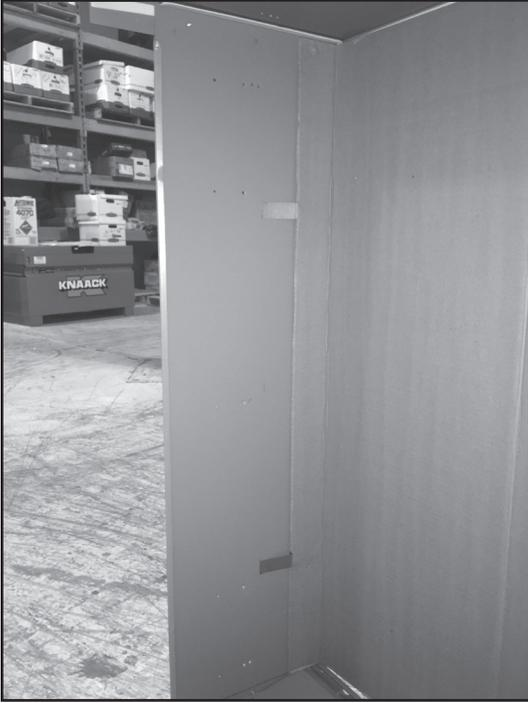
7. Tape the top, bottom and side of the insert to insure that the least amount of outside air can get behind and dislodge the insert.
