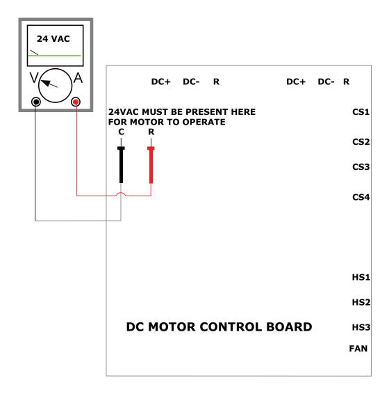
**LEAVE ALL CONTROL WIRES ATTACHED DURING TEST**
