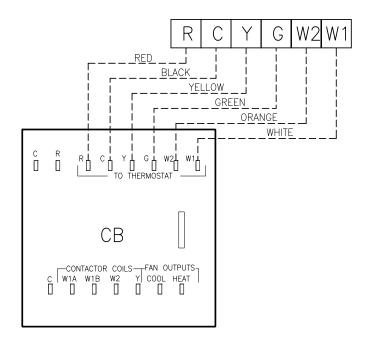
**Note:** If a 2 stage thermostat is not used connect both white(w1) and orange(w2) wires together.
