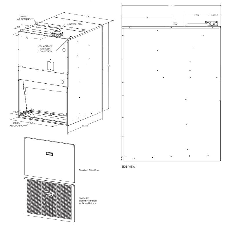
NOTE: Unit must be mounted a minimum of 8 inches above finished floor.
