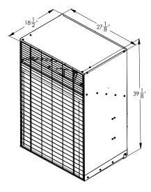
**Note:** Some dimensions that are shown in these drawings are measured between the edges of screw heads.
